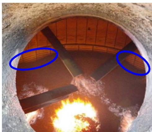
**Fig.1.** Concave shape on the burden surface beneath the probes
